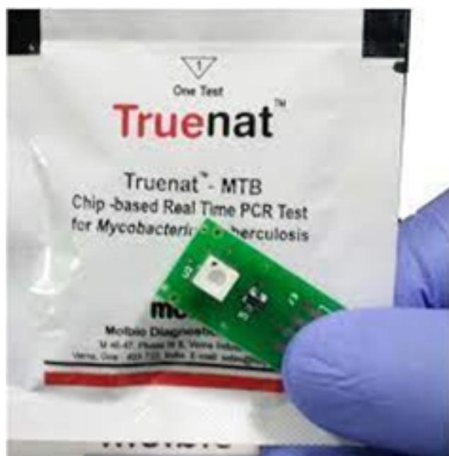
**Fig. 3:** TrueNat MTB chip (Reprinted from molbio diagnostics product listing [https://www.molbiodiagnostics.com/product\\_details.php?id=1](https://www.molbiodiagnostics.com/product_details.php?id=1))
