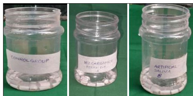
Figure 6: All 3 groups immersed in distilled water for 24 hours
