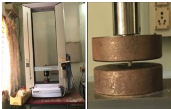
Figure 8: Compressive strength test
