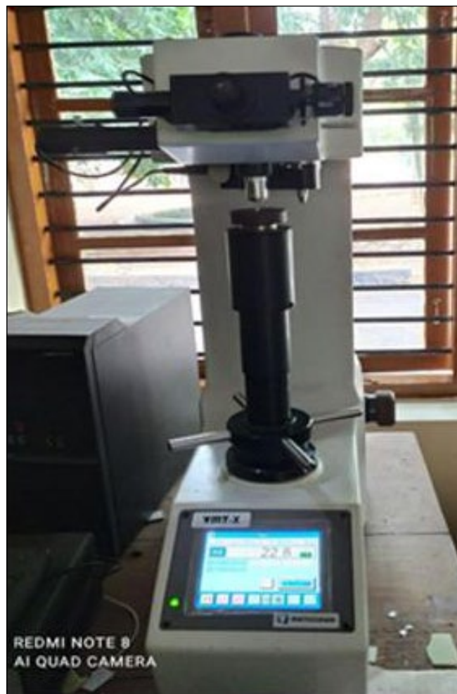
Figure 7: Vickers hardness test
