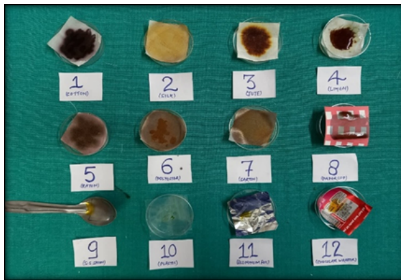
Fig. 6: Group A 4 : Study items subjected to 0.5 ml of lugol's iodine solution after a period of 7 days and colour change is noted.
