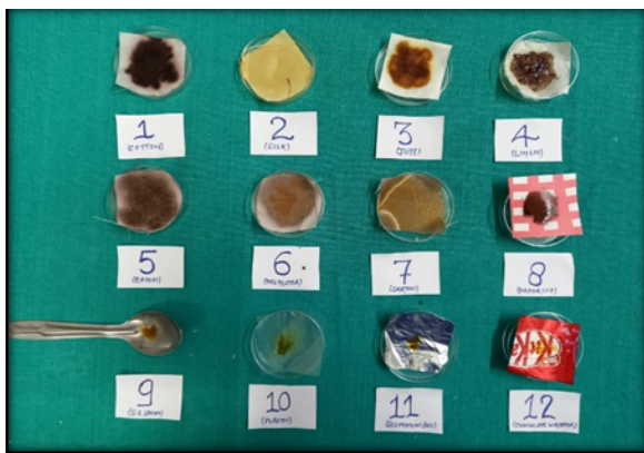
Fig. 7: Group B: Study items washed thoroughly with distilled water allowed to dry at room temperature & then subjected to Lugol's iodine and colour change is noted.
