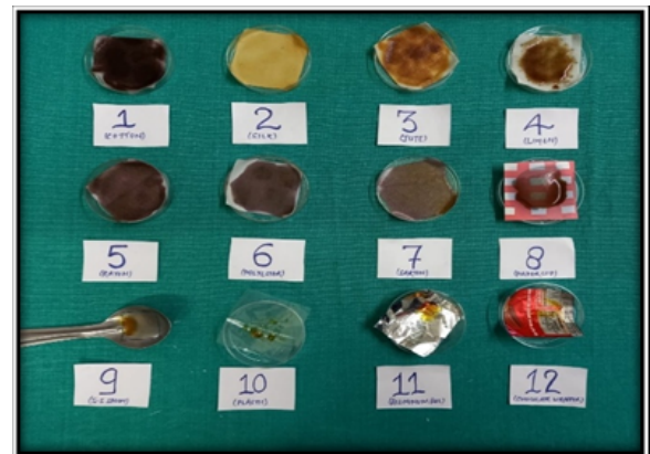
Fig. 3: Group A 1 : Study items subjected to 0.5 ml of Lugol's iodine solution after a period of 12 hours and colour change is noted.
