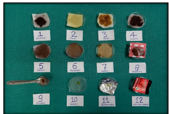
Fig. 9: Group D: Study items washed thoroughly with detergents (1 gm of commercially available detergents Tide to be mixed in 500 ml of water) allowed to dry at room temperature & then subjected to Lugol's iodine solution and colour change is noted.
